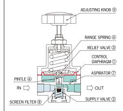
Range spring ④, which has been compressed by Adjusting knob ⑤, causes Pintle ⑥ to move downward,opening Supply valve ② and allowing air flow to the downstream.The pressure builds up against Control diaphragm ① until Supply valve ② closes.
